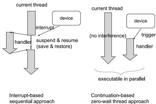
**Figure 1. Two different approaches in handling external events from devices.**
