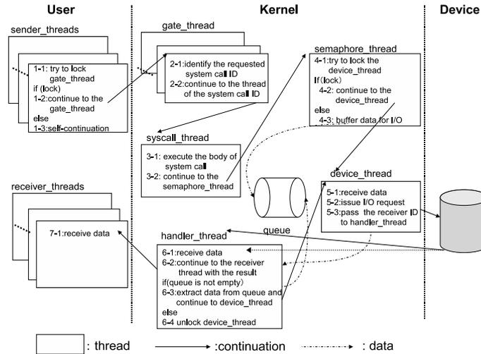
Figure 4. Handling multiple I/O requests with zero-wait threads.
