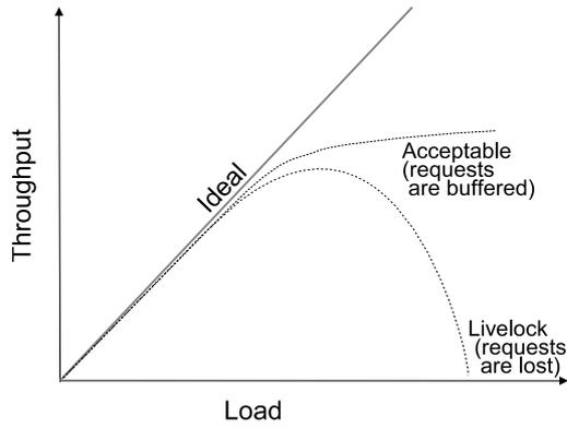
**Figure 6. Overloaded systems may lead to receive livelock in which no useful work cannot be performed.**
