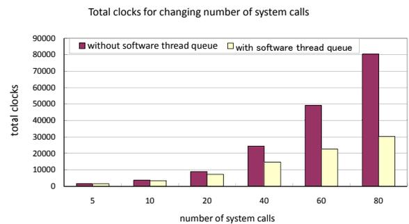
**Figure 11. Comparison of total clocks in changing number of system calls before/after using software queue**
