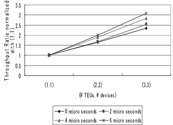
**Figure 5. Relative throughput normalized compared to the case (the number of devices, the number of TEUs) is (1, 1).**
