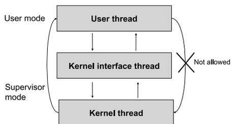
**Figure 2. Mode changes between threads in the FUCE processor.**
