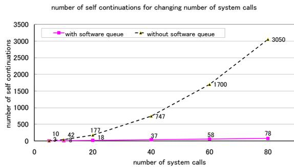
**Figure 10. Comparison of number of self-continuations in changing number of system calls before/after using software queue**
